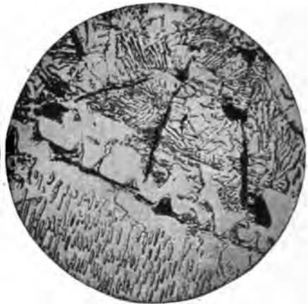
FIG. 181.—Mottled Cast Iron. Magnified 500 Diameters. (Wust.)
